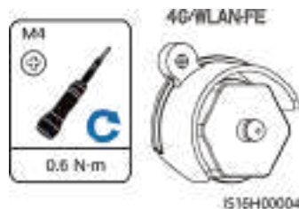
Figure 5-44 Installing anti-theft components for the Smart Dongle
