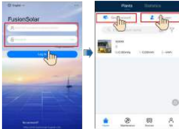
Figure 7-5 Creating a PV plant and a user
