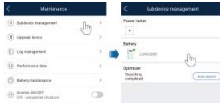
Figure 7-13 Adding a battery
