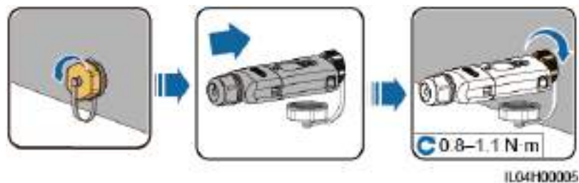
Figure 5-10 Installing a WLAN-FE Smart Dongle (WLAN communication)
