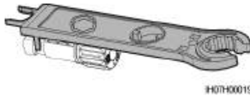
Figure 5-14 Removing a DC connector
