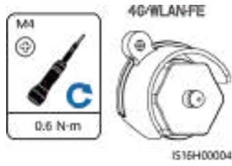
Figure 5-49 Installing anti-theft components for the Smart Dongle
