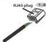
Figure 4.36 Strip the insulation layer and connect to RJ45 plug
