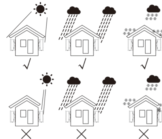
Figure 5.1 Recommended Installation locations
