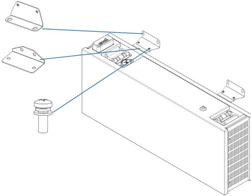
**Step 3:** Stack the installed batteries on top of the already placed base.
