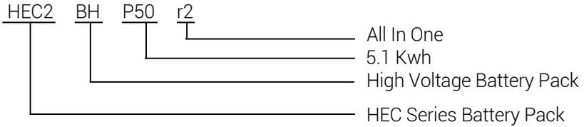
HEC2-BHP50r2 can be used in conjunction with inverters and can store and release electrical energy according to the requirements of the inverters.
