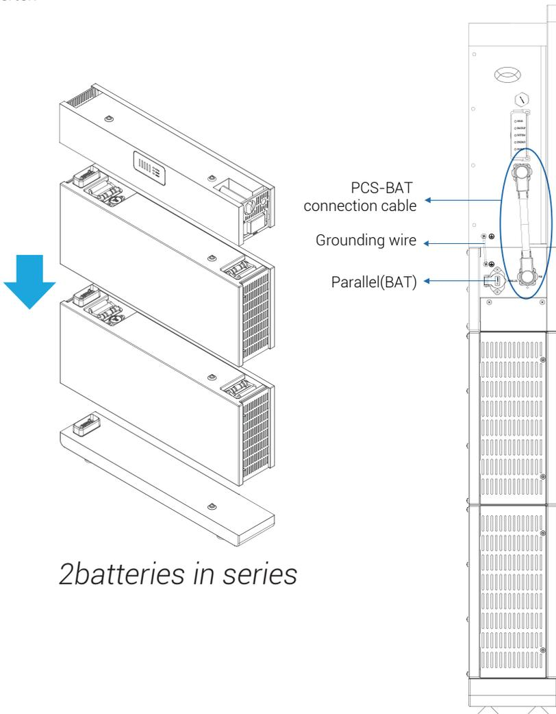
1.If you want to install the HEC2-BHP200r2-A ,HEC2-BHP300r2, HEC2-BHP400r2 series battery packs, you need to connect cable to the parallel ports of the two BMS main boxes.
