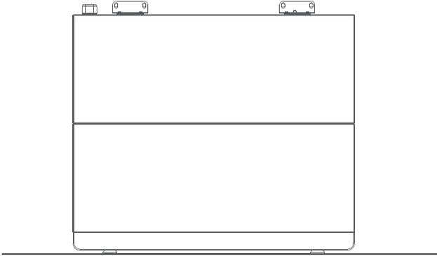
**Step 7:** After installing the battery module, place the high-voltage box on top of the battery box. Please align the high-voltage box with the front of the lower battery during installation.
