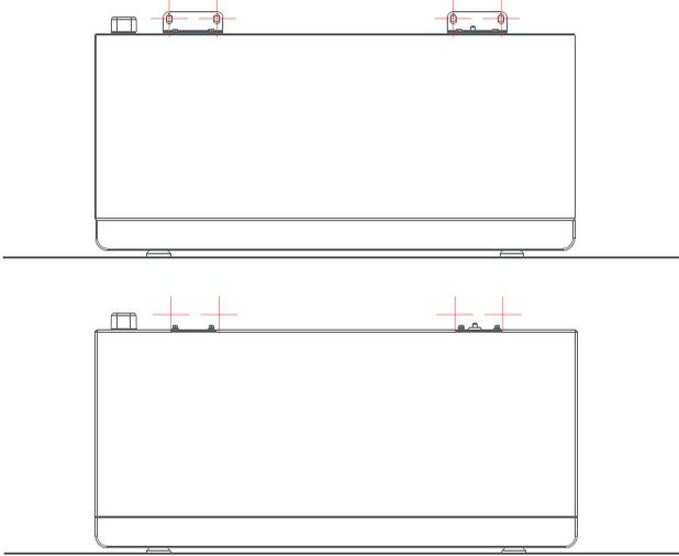
**Step 5:** Install expansion bolts in the drilled holes. Use the expansion bolt with its own M8 nut to fix the wall battery pendant with the expansion bolt. Afterwards, use four cross recessed pan head screws with M5x14 to fix the wall battery mount and pack mount.
