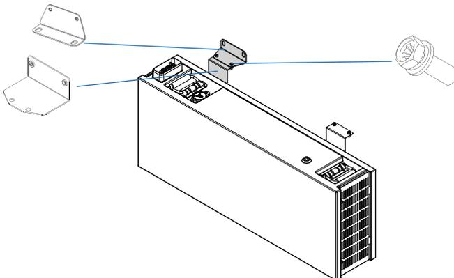
**Step 3:** Use four phillips head screws and a three M5x14 unit to install the battery pack, and wall battery mounts. As shown in the following figure.
