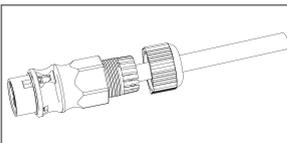
Tighten the nut with an open-ended wrench
