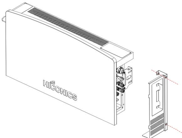
**Step 2:** Place the inverter on the BMS main box, fix the inverter on the mounting bracket, adjust the whole system, and ensure that the battery and inverter are firmly hung on the panel and bracket.
