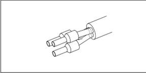
Crimp the terminals with crimping pliers
