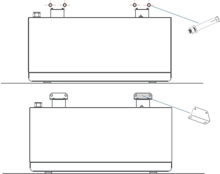
**Step 6:** Repeat steps 2 to 5 to install the other battery modules required. Please align the lower battery with the front of the upper battery during installation.
