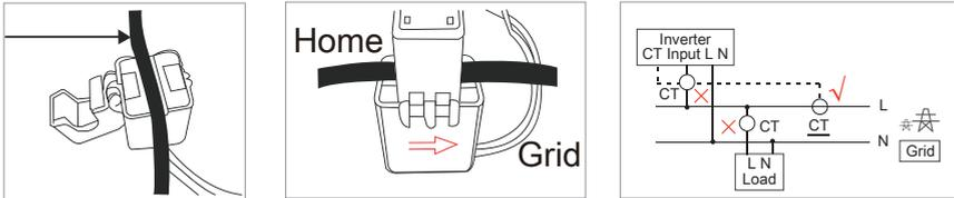
4. Connect the S1 and S2 cables of the CT to the RJ45 adapter, and connect the wires as shown in the diagram.
