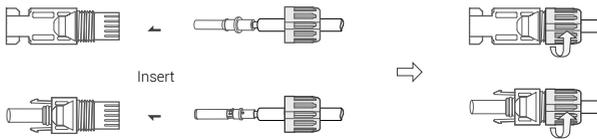
**Step 5:** Plug the PV connector into the corresponding PV connector on inverter.
