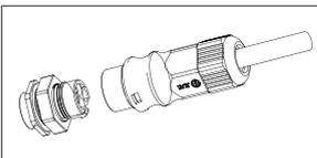
The installation arrow indicates insertion the male connector
