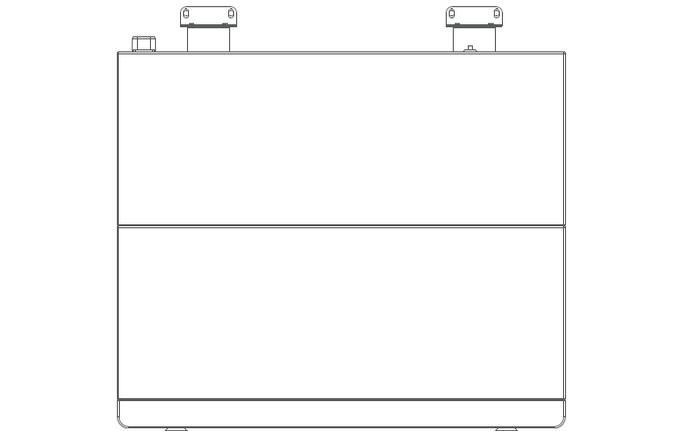
**Step 7:** After installing the battery module, place the BMS control box on top of the battery box. Please align the BMS control box with the front of the lower battery during installation.
