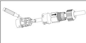
Crimp the wire with a hexagonal screwdriver and turn the screw. torque  $1.2+/-0.1\text{N}\cdot\text{m}$  ( $2.5\sim 6\text{mm}^2$ )
