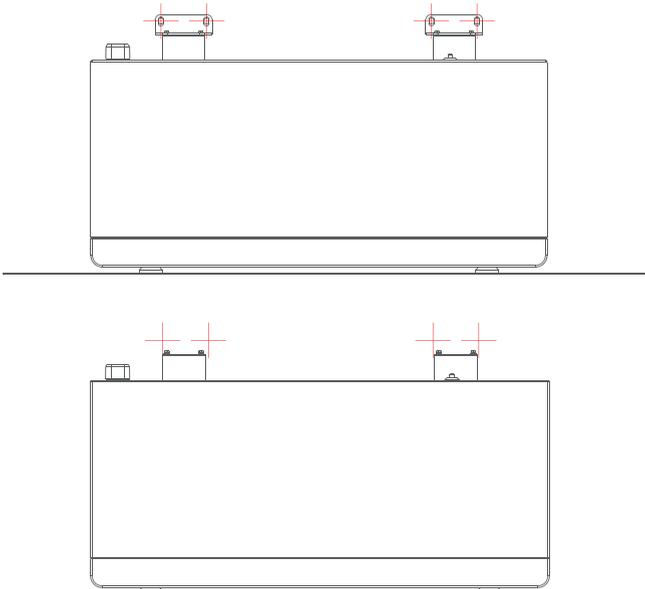
**Step 5:** Install expansion bolts in the drilled holes. Use the expansion bolt with its own M8 nut to fix the wall battery pendant with the expansion bolt. Afterwards, use phillips head screws head screws with M5x14 to fix the wall battery mount and pack mount.
