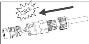
Insert the main body into the rubber core and hear the "click" sound
