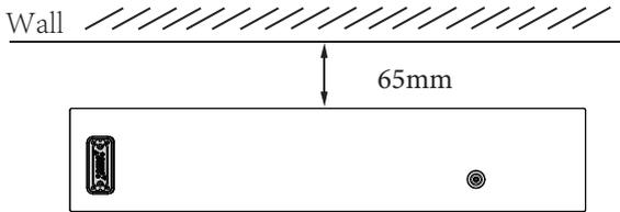
**Step 2:** Use four phillips head screws and a three M5x14 unit to install the battery pack, and wall battery mounts. As shown in the following figure.
