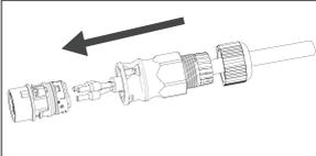
Set the parts on the cable, Insert the terminal holes in sequence
