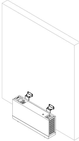
**Step 4:** Use a marker to draw dots at the red intersection in the following image. After drawing the dots, remove the wall battery pendant and use a drill bit to drill holes.
